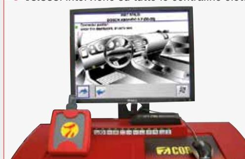
*Cal One-Touch, steering wheel rotation sensor calibration system integrated in the wheel aligner. Essential for correctly aligning wheels on cars equipped with ESP, adaptive suspensions, dynamic steering, electric power assisted steering and adaptive lighting systems.*
