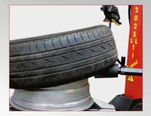
**TAPERED ROLLER**. Facilitates demounting and mounting of first bead by keeping the bead within the rim well. **Facilitates demounting of second bead**.
