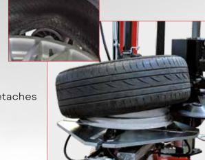
The **LARGE DISC** lifts the tyre and detaches the lower bead.
