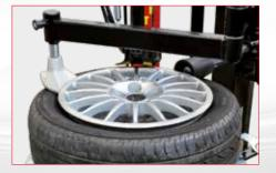
Follows the tyre radially during mounting and demounting and depresses the bead with a roller or, in the case of the WDK version, a disc.
