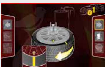
Match-Mounting procedure (rim-tyre)
