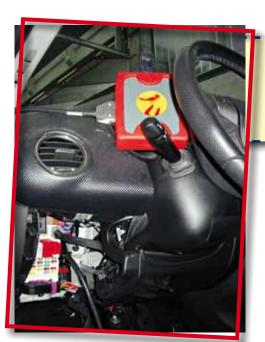
Module for communication with the vehicle's electronic control units.
