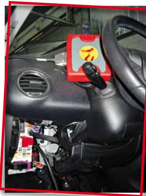
Module for communication with the vehicle's electronic control units. Connection is via the EOBD2 port, which also supplies power to the module.
